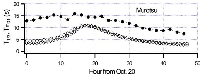
**Fig. 11. Comparison of observed wave periods with forecasted and hindcasted**
