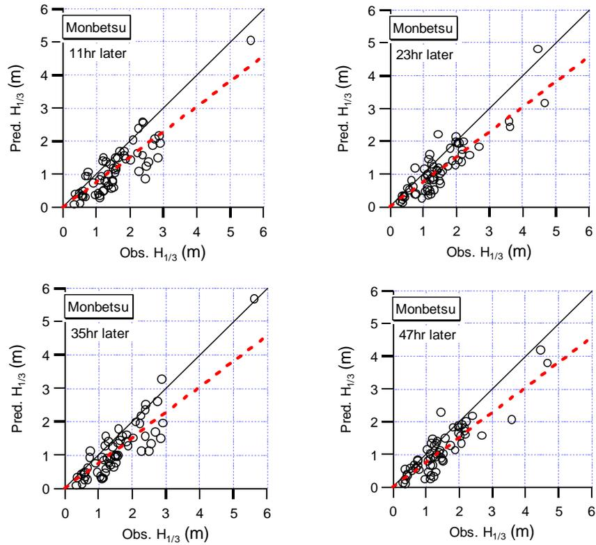
**Fig. 7. Comparison of wave heights with observations**
