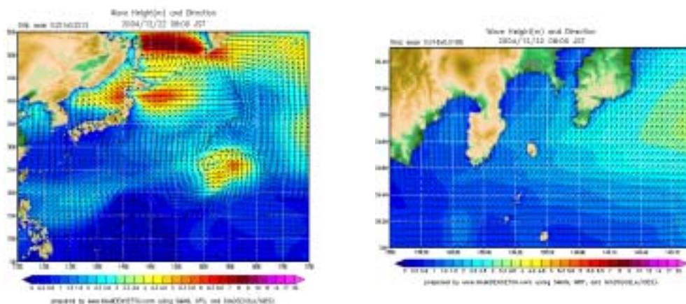
**Fig. 3. Forecasted wave heights and directions for outer and nested domains**
